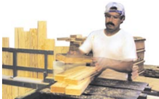
A worker produces pine studs using wood from a landfill.
